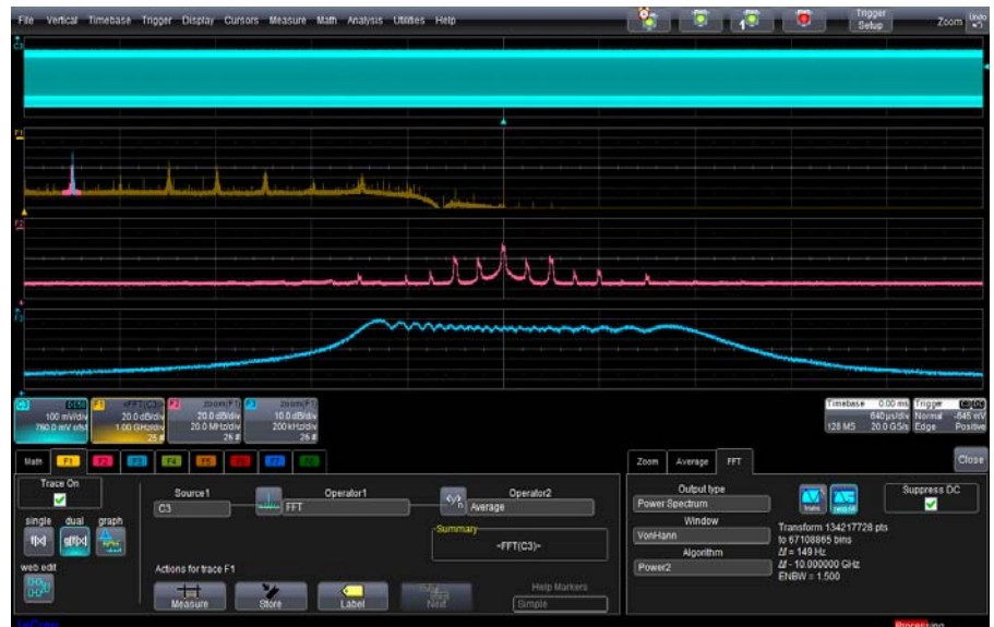
Figure 1 Spectral analysis of a 500 MHz frequency modulated carrier using a 128Mpoint FFT for good resolution bandwidth.
