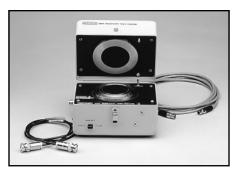
8009 Resistivity Chamber is compliant with American Society for Testing and Materials (ASTM) Standard D 257 Standard Test Methods for DC Resistance or Conductance of Insulating Materials. The 8009 combined with the 6517B provides a complete system for making high quality, safe resistivity measurements.
